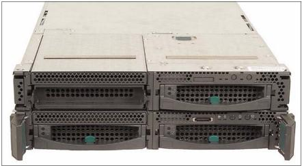
Figure 28: PRIMERGY BX630 scalable server blade (4-way configuration
